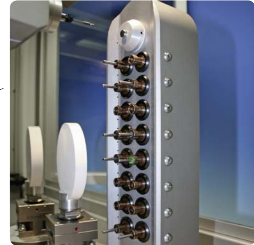
Tool holder, consisting of 16 plug-in-positions and a linear dimension switch-key, used to measure the exact tool length and for breakage inspection.
